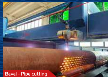
Bevel - Pipe cutting
