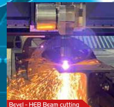
Bevel - HEB Beam cutting
